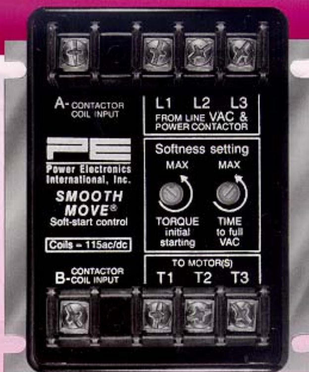
Pictured - SM5A1S - 208 thru 480 vac - 5FLA - smooth control for one or multiple a.c. 3-phase motors up to the rated FLA. 4" x 3-3/4" x 3-3/8" less than 1 lb. UNIVERSAL VAC INPUT allows for easy stocking and wiring!
